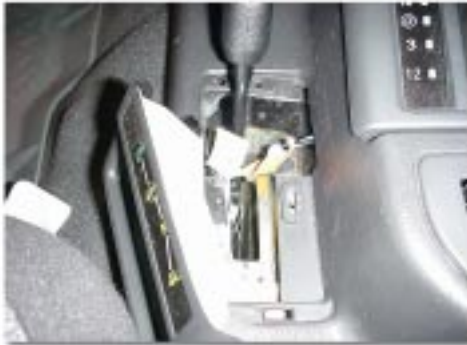
The photo (right) shows the Jeep console removed and the transfer case linkage removed
