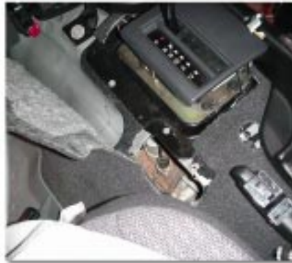
The photo (right) shows the Jeep console removed and the transfer case linkage removed
