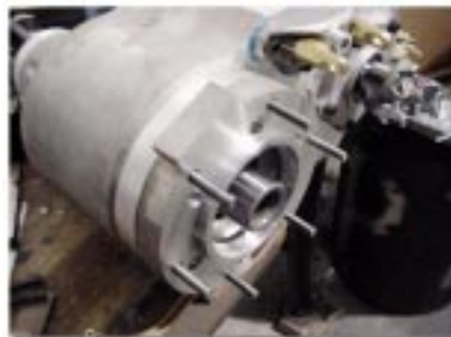
The photo (left) shows the rotation we used to obtain the proper shifter clearance.
