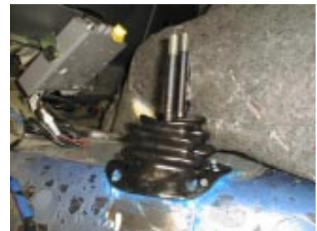
The Atlas boot and handle assembly installed. The carpet must be modified to fit over the shifter assembly.
