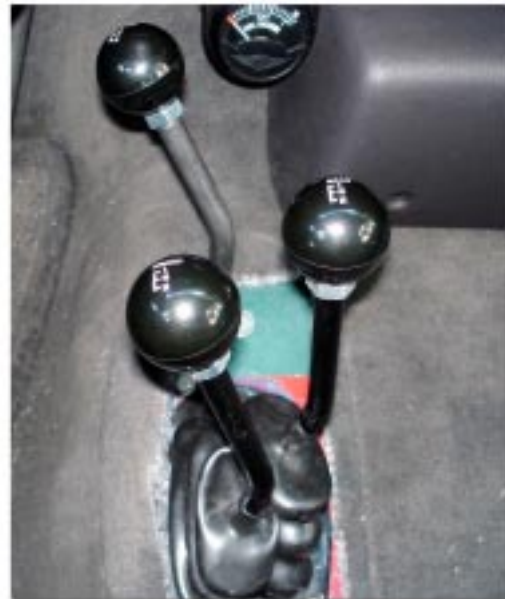
ABOVE: THE STANDARD ATLAS SHIFTERS MOUNTED BEHIND THE PLANETARY CABLE SHIFTER IN A DODGE 2500.
