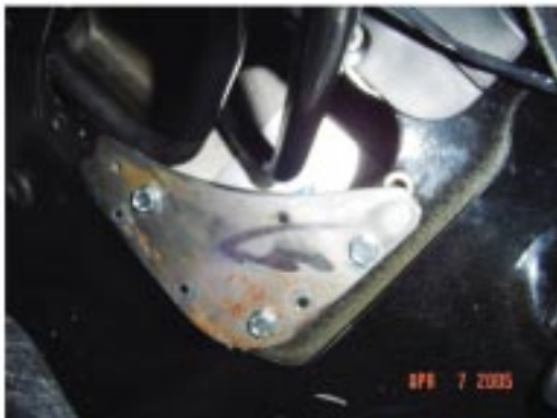
The stock floor mount (shifter and linkage) is removed before initial installation. The console and driver's seat should also be removed for ease of installation.
