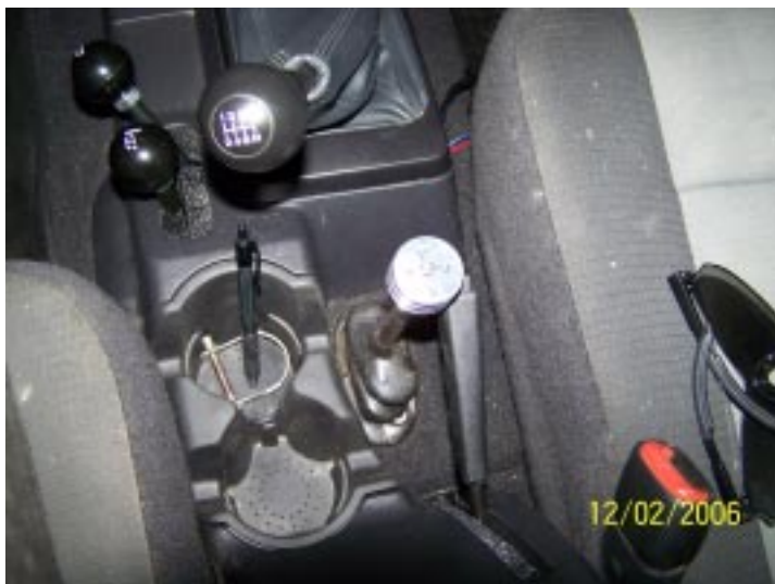
Atlas 4 speed with the reduction shifter installed next to the emergency brake.
