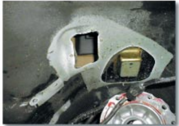
The stock floor mount (shifter and linkage) is removed before initial installation. The console and driver's seat should also be removed for ease of installation.
