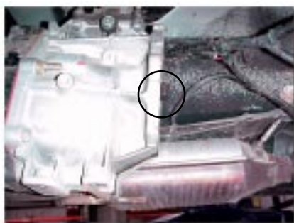
AX5 should have 1/2" output shaft stickout.
