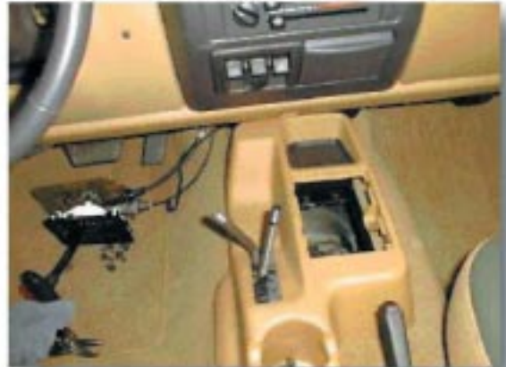
The stock floor mount (shifter and linkage) is removed before initial installation. The console and driver's seat should also be removed for ease of installation.
